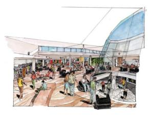
Our design incorporates skylights with operable windows, low speed high volume fans, 100% outside air cycling,  $CO^2$  monitoring, north facing skylight to provide daylighting and a relief path for the 100% outside air cycling.
